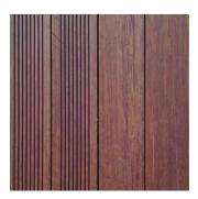
Surface of MOSO\* Bamboo X-treme\* with different maintenance and cleaning scenarios: weathered, dirty decking (left), weathered, cleaned decking (middle), and re-oiled decking (right).
