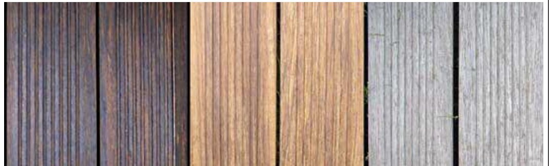
Original colour and colour after some time without maintenance.
